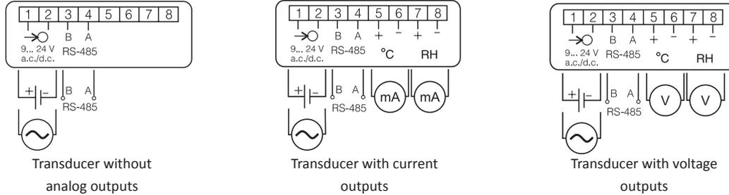
Fig. 1 Connection way of electric signals – P18.
