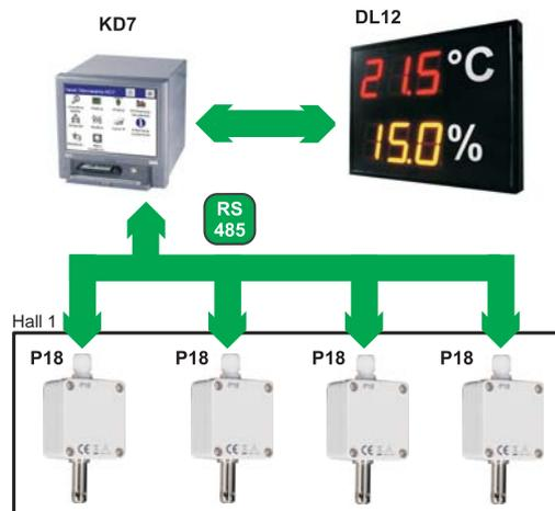
Measurement and recording of temperature and humidity.
