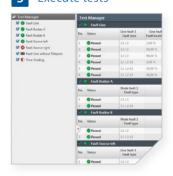
All test steps are executed automatically in a row, even with multiple distributed CMCs. Based on the time grading of the protection system, the trip times can be autoassessed.
