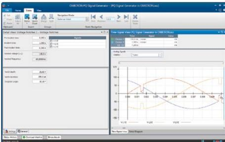
Another example of the module's versatility is the generation of cyclic notches. The notch depth and the angle of occurrence can be adjusted independently; the minimum gap-width for notches is 300  $\mu$ s. This function can provide the possibility to simulate the system perturbation of a thyristor-controlled motor.
