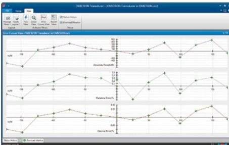
The “manual test” mode is used, if a measurement transducer is to be re-adjusted. Every desired input quantity can be generated for the transducer. Furthermore, it is easy to switch between significant points of a characteristic, where the error of the transducer is shown at a certain input value.
