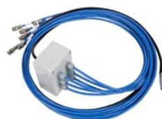
This connection cable with Twin-BNC clamp plugs type AMPHENOL 31-224 is tailored to connect ABB relays of the REF 54x series (with AMPHENOL Twin-BNC bulkhead receptacles type 31-223) to the low level outputs of a CMC test set (16-pole LEMO connector). Cable length: approx. 2.5 m (8.2 ft). The six cable tails with the AMP connectors are labeled.
