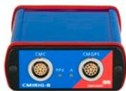
CMIRIG-B is an interface box enabling the connection of devices sending or receiving the IRIG-B protocol or PPS signals with CMC test sets<sup>1</sup>. CMIRIG-B performs the level conversion between the CMC and the sources or receivers. The actual IRIG-B decoding and coding functionality is implemented in the CMC test set. CMGPS 588 can optionally be used as PTP Grandmaster Clock in order to establish a link to absolute UTC time.
