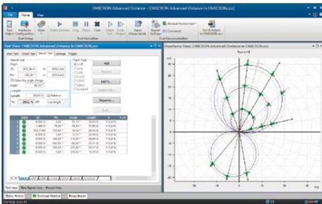
A test in Advanced Distance can have any combination of Shot, Search, or Check tests. At test execution, the whole test settings are executed sequentially. This versatile system offers a wide range of testing possibilities. Using this, it is easy to comply with most different testing philosophies and regulations.
