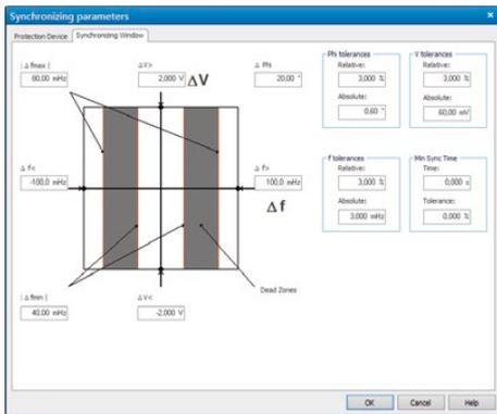
The software automatically detects the circuit breaker closing command from the synchronizing device or synchro-check relay and, taking the CB closing time into account, evaluates if the synchronization takes place inside the synchronizing window. The control of the second output is variable following different test modes. The frequency and amplitude can be changed linearly depending on the ramping time constants of the generator.
