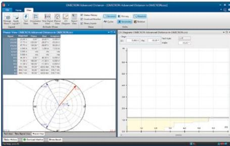
Adding test points and test lines to the tables is possible in a variety of ways. Parameters can be precisely defined by numerical inputs, or specified directly in the characteristic diagram. A magnetic cursor supports the choosing of meaningful values. Mouse commands, context menus and keyboard shortcuts facilitate data input.
