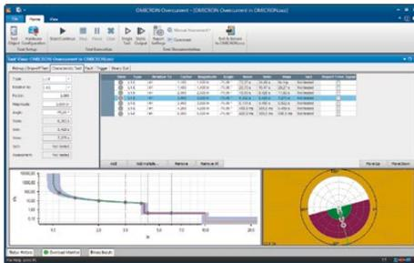
The software overlays the characteristics of each of the elements in both the I/t diagram and the directional diagram. This includes all of the elements which respond to the type of fault applied. For each test shot an assessment of the relay's performance is made based on the allowable tolerances for the measurement of the current and the operating time.
