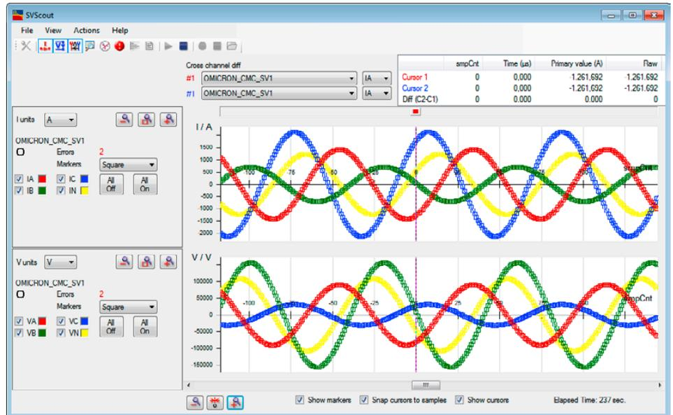
Captured Sampled Values can be saved in COMTRADE files for further in-depth analysis. Expert functions provide even more details on the received data, such as the detailed decoding of the quality codes.
