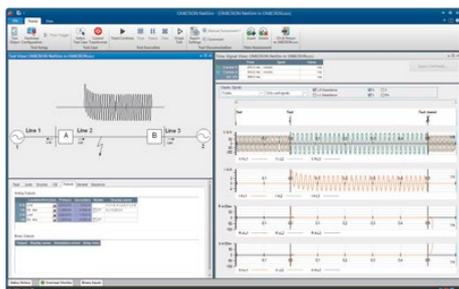
The transient voltages and currents are calculated from a digital network model, providing an optimal approximation of the real events in a power network. CT saturation may be simulated using real CT excitation and burden data for each measurement location. This data could, for example, be measured on site with the OMICRON CT Analyzer.
