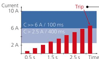
With the Pulse Ramping module the determination of the  $I >>$  pickup value is possible because the 200 ms pulses do not force a trip in the  $I >$  region.
