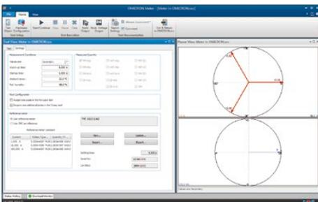
In a detail view, all parameters can be specified independently for each phase. Apparent, active and reactive power is indicated for each phase and the whole rotary system. Testing of the following meter functions is supported:
