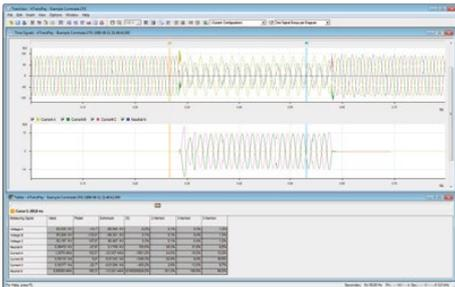
For the analysis of a transient recording, amplitude and time measurements can be performed using two cursors. The voltage and current values on the cursor positions are displayed in the vector diagram or the value table. In every view, the zoom function allows the representation of the values with optimal scale. TransView allows for simultaneous analysis of multiple recordings, e.g. of the two ends of a line.
