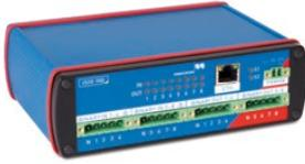
ISIO 200 is a simple and versatile binary I/O terminal for Substation Automation Systems (SAS). It communicates via IEC 61850 GOOSE messages and, therefore, interoperates with CMC test sets supporting GOOSE and a wide range of intelligent electronic devices (IED). ISIO 200 is configured via a built-in web interface and no special configuration software needs to be installed.
