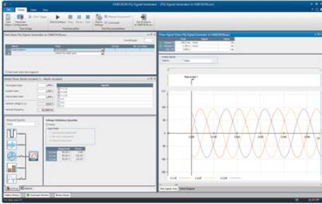
The need to verify the capability and reliability of power quality meters/analyzers requires appropriate calibration equipment. The PQ Signal Generator turns a CMC test set – ideally a CMC 256plus with its high-precision voltage and current outputs – into a calibration tool that generates all kinds of power quality phenomena according to IEC 61000-4-30 (-7, -15):
