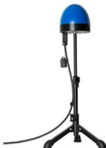
The CMGPS 588 synchronization unit is an antenna-integrated GPS controlled time reference optimized for outdoor usage. It works as a Precision Time Protocol (PTP) Grandmaster Clock and does not require any configuration work. It is automatically ready for operation within a very short time after providing power supply via Power over Ethernet (PoE). The distance between the CMGPS 588 and the CMC can be extended up to 95 m (312 ft) by using extension cables.
