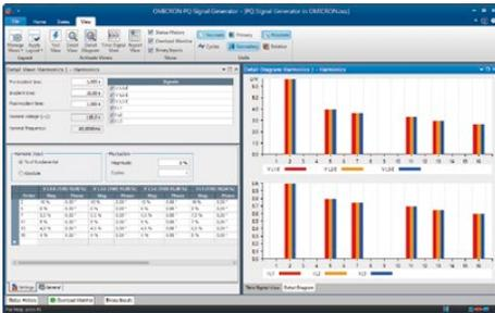
The PQ Signal Generator provides a powerful and easy to use interface; for example, flicker signals with rectangular or sinusoidal modulation can easily be generated. Flicker magnitude and flicker frequency starting from 1 mHz can be set individually by the user.
