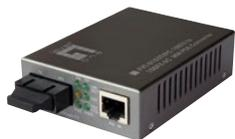
This converter connects a CMC or a DANEO 400 to a network via fiber optics. The 100TX to 100FX-SC Converter transfers data from a 10/100Base-TX copper to a fiber interface. It is designed to receive both data and power from PoE networks, and to pass on the data to a fiber optics connection.
