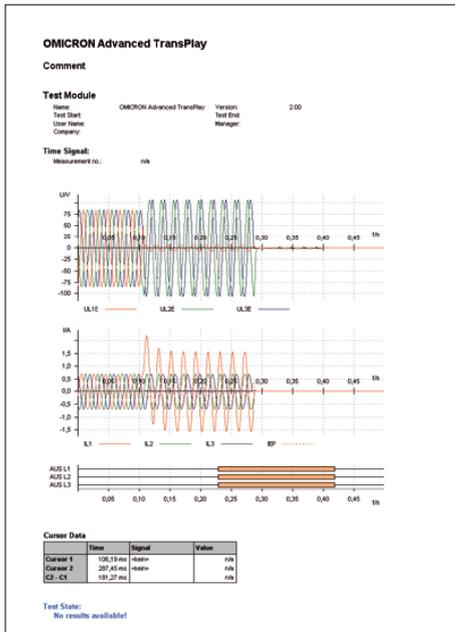
Besides playing back voltage and current signals, Advanced TransPlay can also replay the binary signals in a fault recording via the CMC's binary outputs. Additional binary signals (e.g. carrier send/received signals from communication-based schemes) can be added. During playback, the selected voltage, current, and binary signals are applied to the protection device. Playback can be synchronized via GPS, IRIG-B protocol or by a time pulse applied to a binary input.
