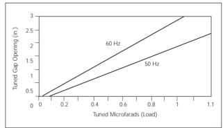
Resonating Inductor gap opening vs tuned load
