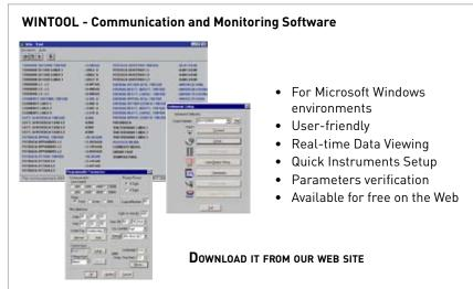
WINTOOL software enables the power meters to be connected to a PC for measured data viewing. It allows an easy and fast way to set the instrument parameters by a desktop or portable PC.
